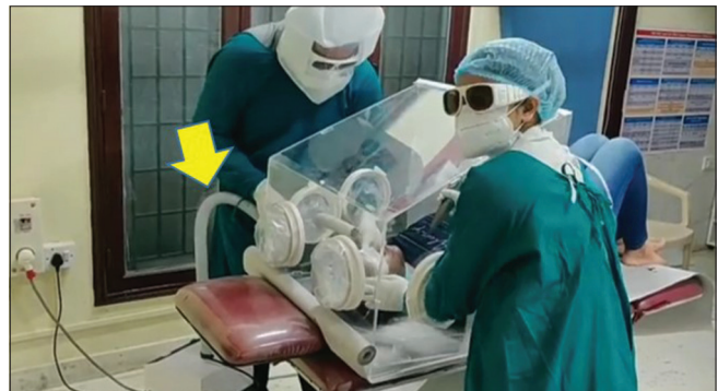
Figure 3: Hood being used for laser toning of the face. Smoke evacuator nozzle (yellow arrow) and part of the hose is kept inside the hood near the area being treated
